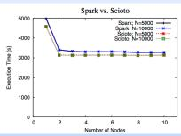
All benchmarks were run for 30 steps at the macrosolver level on LANL's Darwin Cluster using 48 cores per node with visualization disabled and the number of grid points specified in the graph. Each grid point contained an MD simulation with 864 particles that converged after 1000 steps. The described Adaptive Mesh Refinement technique was used.
