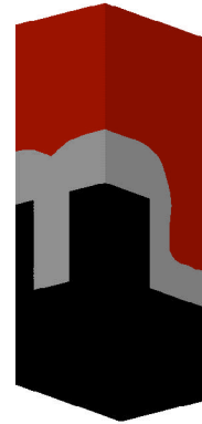
Figure 2. Three region solid geometry model. The two material interfaces are defined by sheet surfaces.
